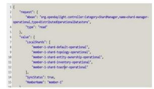
Figure 5 – Yangman JSON output showing mbeans and operational shards.
