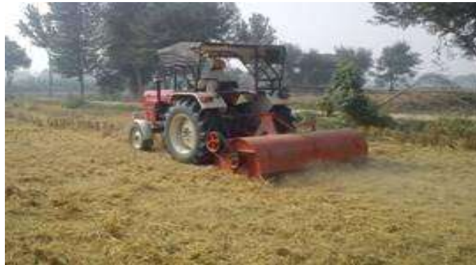
Figure 1: View of paddy straw chopper in operation [3]
