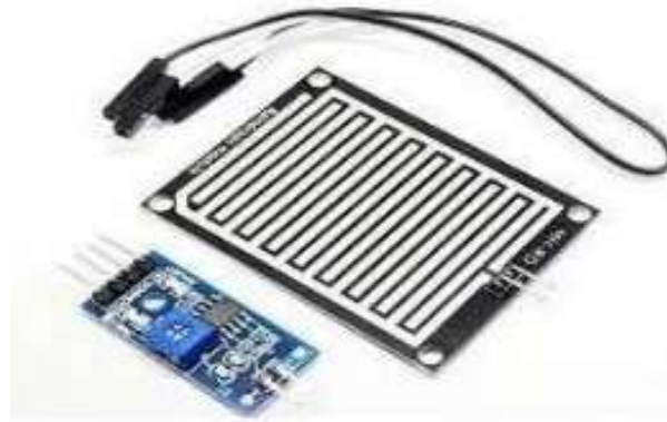
Fig. 1.4 Following Figure shows a Raindrop Sensor Module
