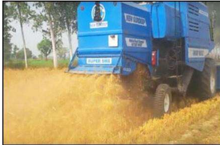
Figure 3: Combine fitted with SMS system in operation [3].
